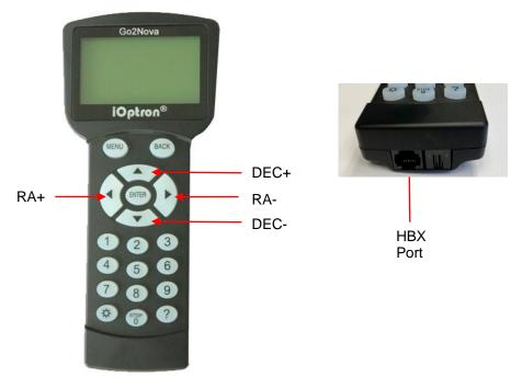
Figure 25. Go2Nova® 8410 hand controller
