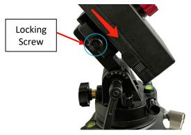
Figure 9 Slide mount head into an EQ base
