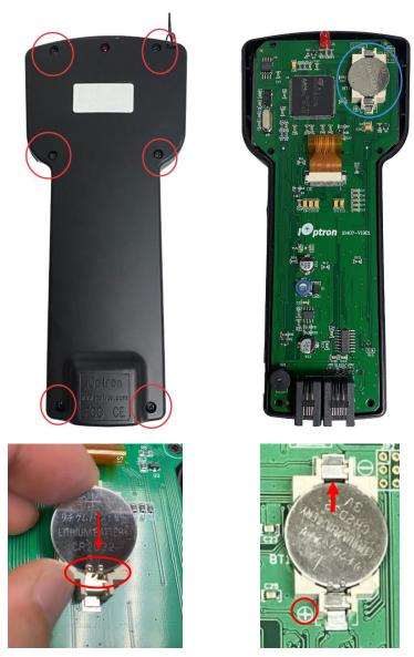
Figure 27. Install a CR2032 battery
