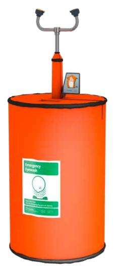
**Maintenance:** Unit must be inspected regularly. Refill unit after testing or use. Water and bacteriostatic additive must be changed at least once every six months.
