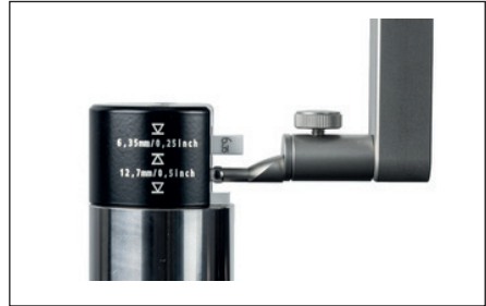
Fig. 13 Positioning the setting gage when calibrating with groove
